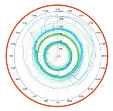
Polar Time Series data is "wrapped" around a 24-hour clock. This allows the user to understand how demand levels change at the same time on different days.
