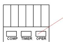
Flash times stand for indoor unit error code(the premise is TIMER is not flashing)
